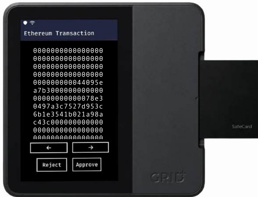
Figure 8: Example Of Structured Transaction Data Displayed On A Hardware Wallet
